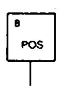
\*HOLD POS DOWN FOR 4 SEC, RCV MODE WILL SWITCH TO STBY IF IN STBY, RCV MODE WILL SWITCH TO PREVIOUS RCV MODE.
